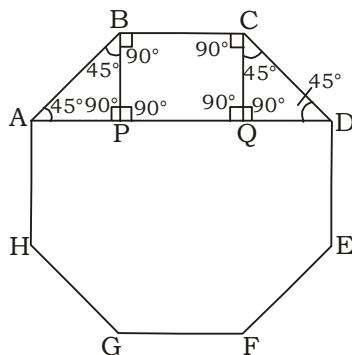
Joining A and D and drawing perpendicular from B and C to AD.
