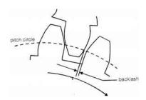
Backlash is defined as the amount by which the width of tooth space exceeds the thickness of the engagement tooth measured along the pitch circle.
