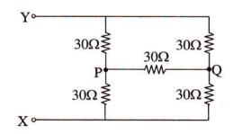
The given circuit is a balanced bridge as shown in Fig.
