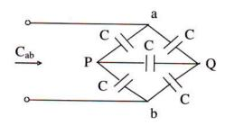
The given circuit is a balanced bridge as shown in Fig.
